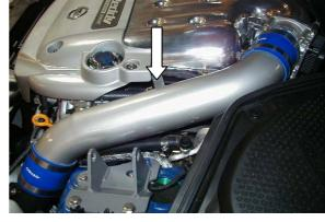
Secure the bracket on C-6 to the Intake manifold
