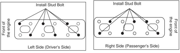
2. Install the Exhaust Manifold using provided gasket and hardware.
