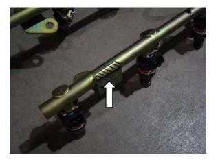
3. Install the 440cc injectors and reinstall the fuel rail using the provided spacer.
