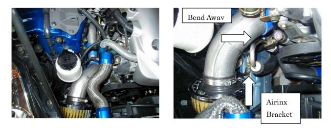
3. Install the S-3 and the S-4 (with AIRINX) to the left (driver side) turbo inlet using provided hose and hose clamps and secure the Airinx to the chassis as shown. Bend the A/C line toward the engine so that the S-4 pipe clears the line.
