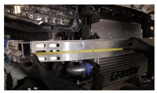
2.5 Drill the two marks that you made with at least a 5/16" drill bit. Make sure you hold the drill level top to bottom and centered left to right when going through the support beam. You may have to step up to a larger size drill bit if you cannot pass the bolt all the way through the support beam.
