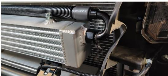
2.12 Install the 6" section of split corrugate tubing to the shorter hose and position closer to the straight hose end. Using the short oil hose, push the hose down and route it the way it is as shown in the pictures below for the easiest fitment. (ITEM #3)
