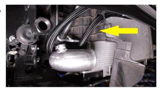
2.11 Route the hose above the oil cooler core. Use grease or oil to lightly lube the threads and o-ring on the 180 degree ORB fitting. This will allow the threads to smoothly spin into the oil cooler core and let the o-ring seat perfectly without tearing. Use a tool to support the aluminum hex port on the oil cooler side, and tighten the ORB fitting into the driver side hole.
